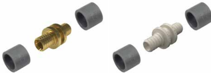
Fig. 50. KAN-therm ultraLINE connector for PEXC, PERT 2 and PERTAL 2 pipes, diameters 14 × 2, 16 × 2,2, 20 × 2,8, 25 × 2,5 mm.
