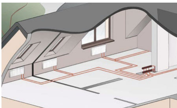
Manifold – tee system in a heating installation
