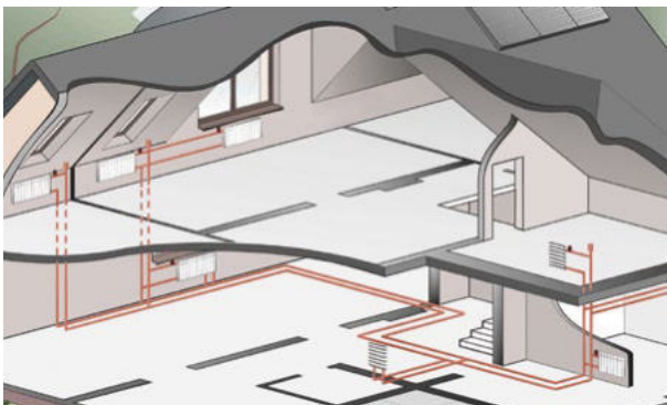
“Vertical” system in a heating installation
