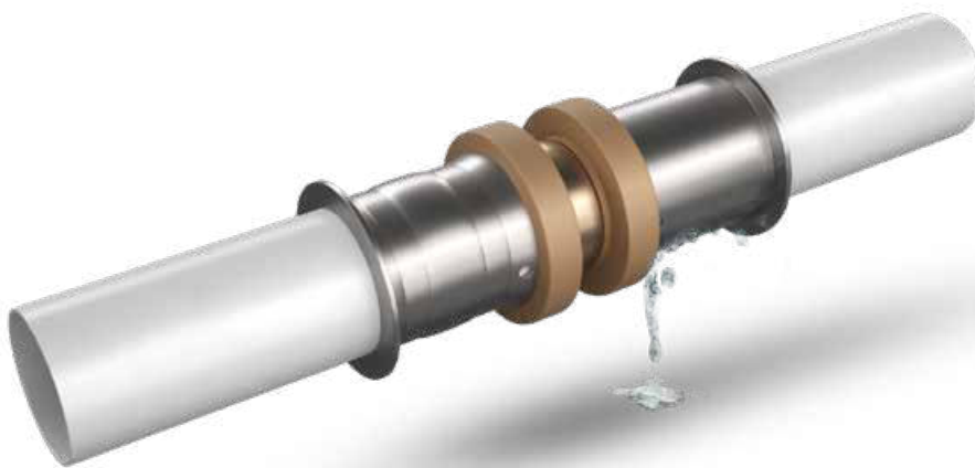
LBP function in action – leak before press
