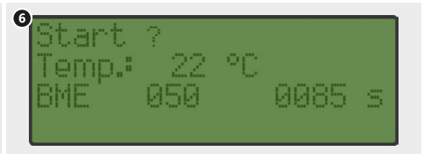
5. Programming of welding machine via laser reader (welding machine will adjust parameters automatically).
