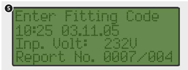
5. Programming of welding machine via laser reader (welding machine will adjust parameters automatically).
